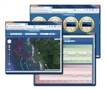
without requiring any additional on-board equipment. Clients can log into the HelmSmart Web site to view live vessel instrumentation while also performing high-speed searches on any vessel network parameter over specified historical intervals. This allows operators to see what a vessel is currently doing while comparing to stored information. For example, current oil pressure readings can be compared against a previous trip for a given engine RPM to determine if a filter needs service.
