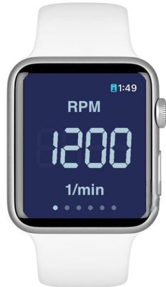
The Apple Watch can directly connect via WIFI or Cellular to a target device's HTTPS or HTTP server after first being configured from the iPhone app.
