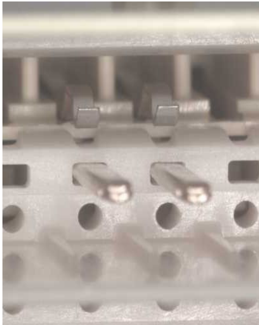
Proper Alignment of Shorting Bar Orientation Feature Un-damaged
