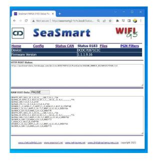
The STATUS CAN link at the top of the CONFIG page can be used to view live PUSHSMART protocol data used for data logging and posting to HelmSmart Cloud services
