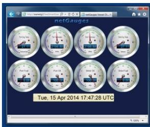
To modify the instrument style and values displayed, select the clock bar at the bottom for additional options
