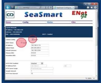
**Step 7:** Enter your new desired static IP address and Router IP address for the Gateway.
