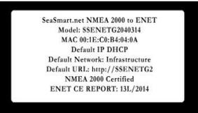
The label on the bottom of the unit will contain the unit's MAC address (unique serial number) and device web URL
