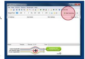
**Step 9c:** After scanning is complete, netScan will report the IP address of all discovered adapters.
