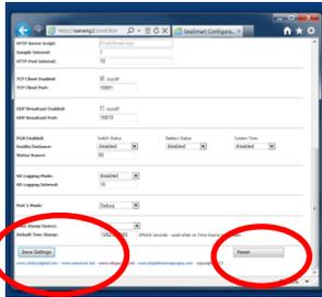
Next select **RESET** to reboot device with new custom configurations.
