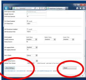
Next select **RESET** to reboot device with new custom configurations.
