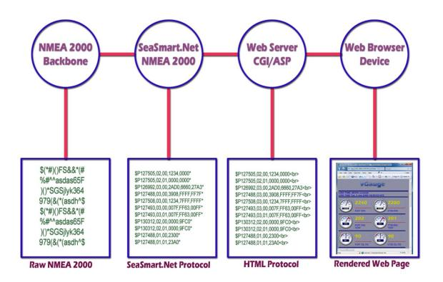
Raw NMEA 2000 data is read directly from the Backbone and translated to SeaSmart.Net protocol so it can be passed on and processed by Web Servers. The Web Servers then in turn format the data into HTML friendly documents which can be retrieved by common Browser based devices. The Browsers render the live data into graphical displays that are easily customizable via standard Web design tools.
