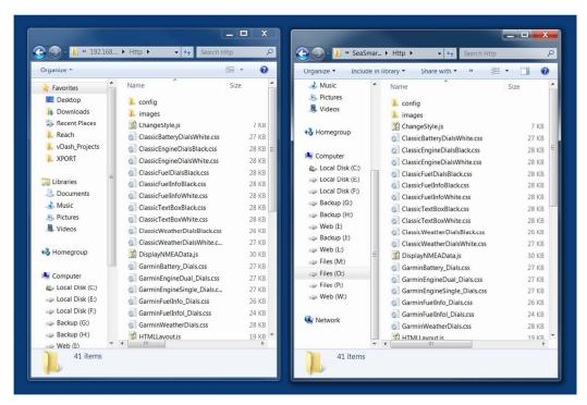
After Copy is complete – verify all files were transferred by viewing contents of directories and checking number of files in each sub directory with source. Occasionally, some files may not be copied due to Flash Compaction timeout. If this occurs, repeat the upload process and confirm file overwrite.
