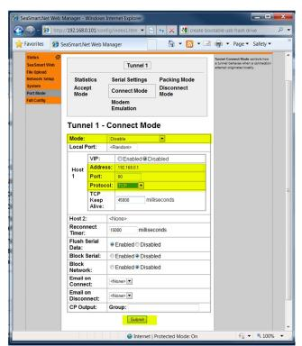
Connect Mode – Web Server Post – Setting the protocol to TCP and Port number to 80 will enable SeaSmart.net to POST data directly to a local Web Server running ASP. The live data can then be logged and viewed with any Browser.
