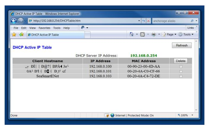
The SeaSmart.Net home web page can be accessed by typing in the IP address into the browser address bar. For example, if the SeaSmart.Net device address is 192.168.0.101, then type http://192.168.1.101. This will load the home page as shown.
