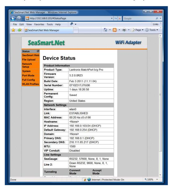
SeaSmart.Net WiFI modules can support multiple WLAN Profiles to allow for auto discovery of configured networks in a fall back boot mode. WLAN Profiles are tried in order until a successful connection is made.
