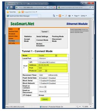
**Connect Mode – UDP Broadcast** – Data is sent to all devices on the subnet using the specified port number. Each receiving device must be set to listen on its on interface IP address. Allows multiple devices to receive the same SeaSmart.net transmissions
