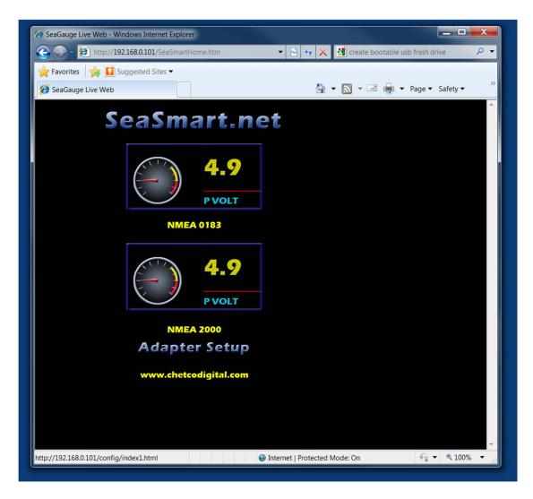
NMEA 0183 \$IIXDR data - SeaGauge Remote Sensor Units output data using NMEA 0183 \$IIXDR sentences and RS232 serial formats. These Web Pages translate and display the data in real-time as it is received from an attached unit.
