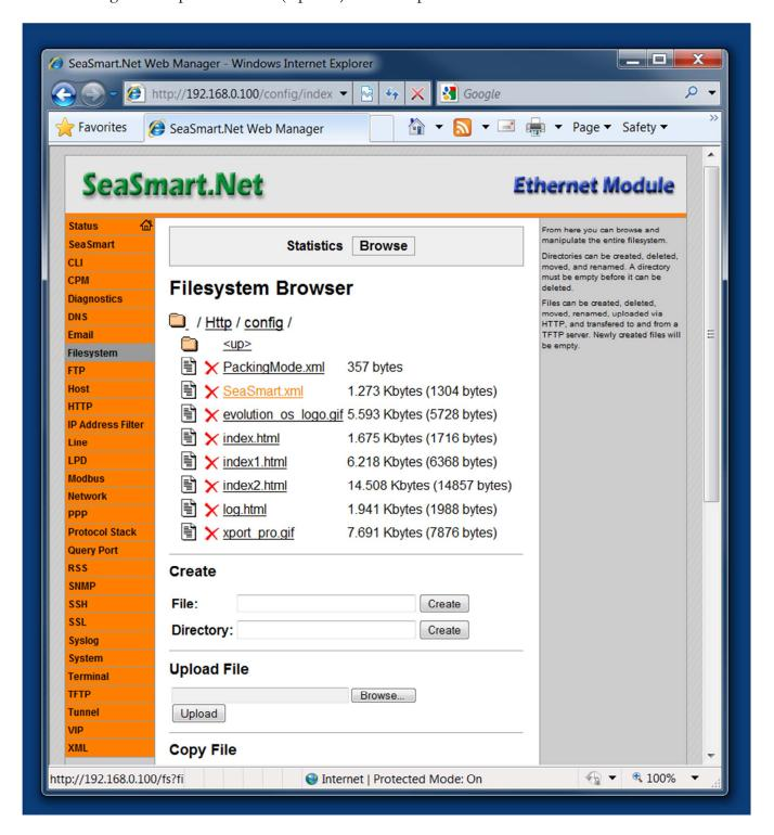
The contents of the SeaSmart.xml file can be read to determine the current operational mode of the adapter. The SeaSmart.xml file can also be modified and reloaded to alter device settings.
