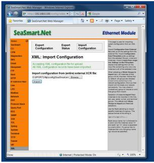
AFTER IMPORT, REBOOT (REPOWER) THE DEVICE TO APPLY CHANGES.
