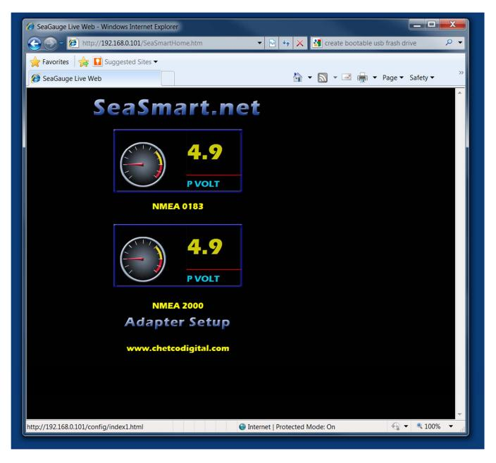
Selecting the ADAPTER SETUP link will navigate to the SeaSmart Configuration page were various set up and maintenance operations can be performed.
