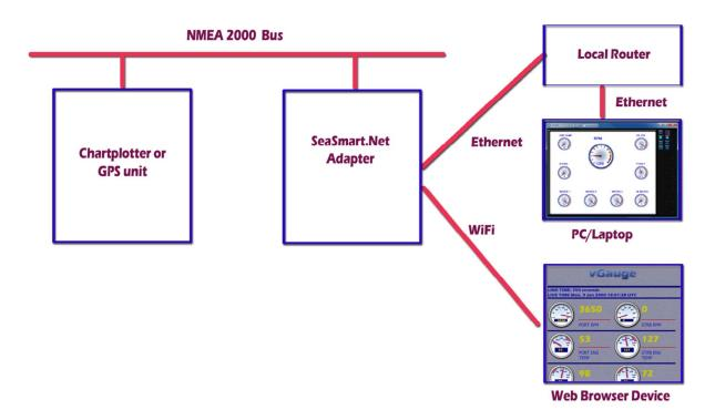
SeaSmart.Net adapters can provide either a wired Ethernet or wireless WiFi connection to a local router (Infrastructure Network). The router then interfaces to other devices on the network via additional wired or wireless interfaces. It is possible and often practical, to use the WiFi features of a local router to service other wireless clients.
