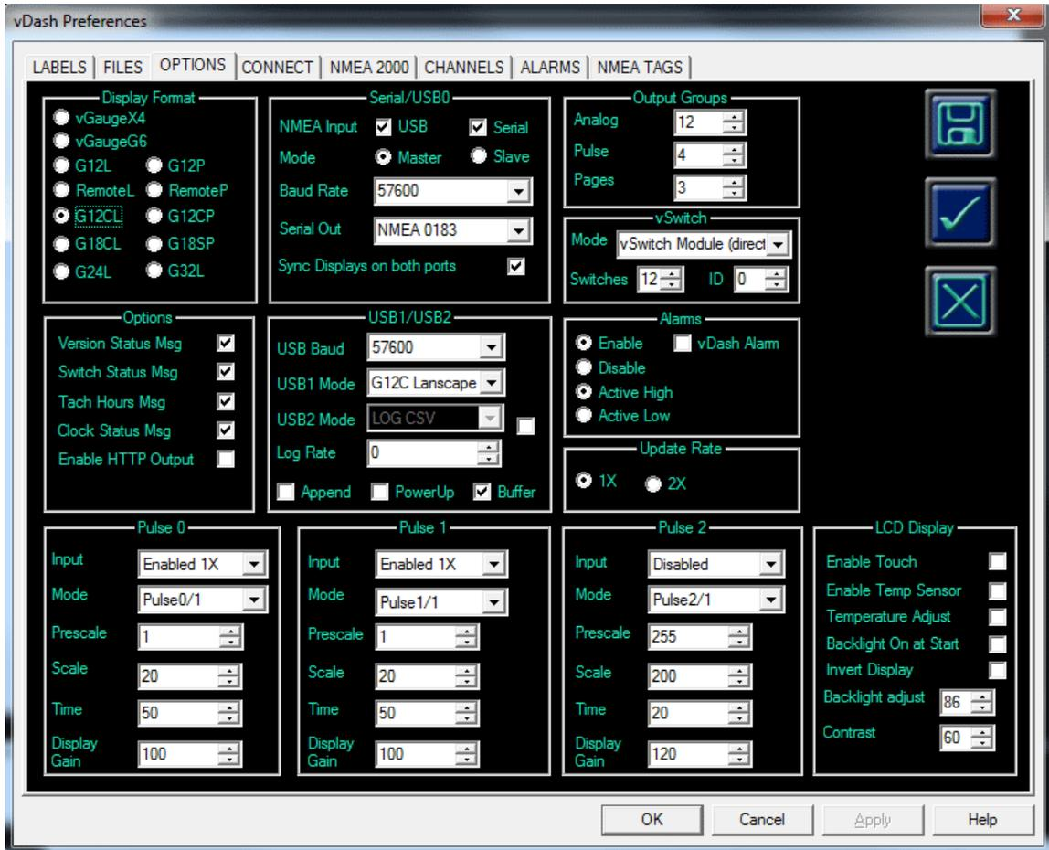
The OPTIONS panel contains several sections for configuration of vGauge/SeaGauge-Remote and vGauge/SeaGauge Display heads. Not all units use the same options so some settings may change depending on selection.
