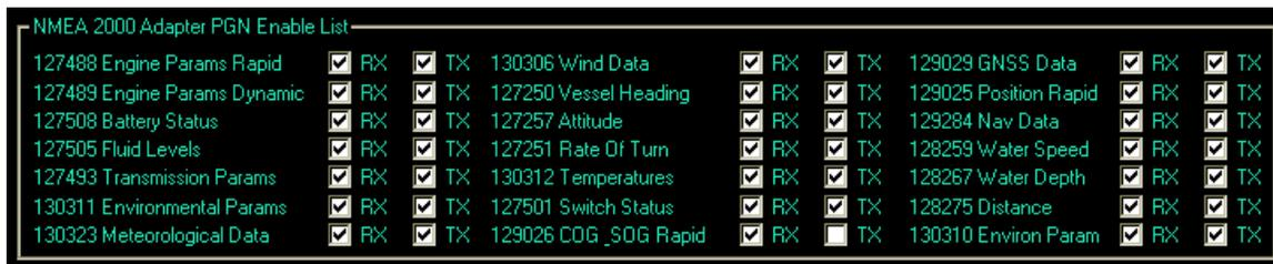
After setting the PGN Enable List, SAVE the changes by using the disk icon in the upper right of the dialog box. The next time a connection is made to the N2K adapter, the new list values will be set and retained.
