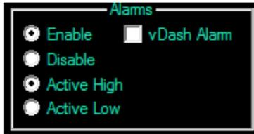
Alarm functions can be globally enabled or disabled by setting the **ALARMS** radio buttons. If driving a pizo alarm directly then choose **ACTIVE HIGH**. Other wise if driving a high current alarm through a relay choose **ACTIVE LOW**.
