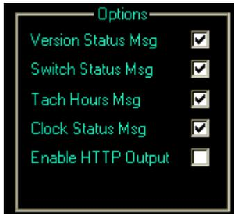
The Options section allows enabling various status messages on the NMEA 0183 output. These messages can be displayed in the vDash title bar used by other connected device.
