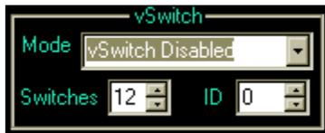
The vSwitch section controls the Switch or Indicator Module attached to the Auxiliary port on the Remote Sensor Unit. The number of Switches or indicators is set from 0-12. The value controls the number of switches or indicators displayed in vDash or Remote display heads.
